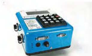
Easily accessible serial ports for external communications. LEDs show data transmittal status. External power supply port. In-line fuse for internal circuitry protection.
