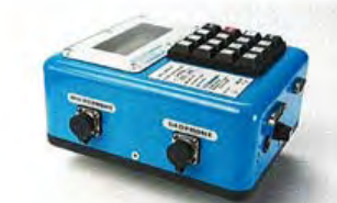
Instrument connection ports come standard with caps to protect connecting pins when not in use.
