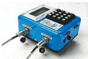
Heavy-duty twist-lock metal cable connections are standard design features on all GeoSonics® seismographs.
