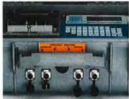
Instrument connection ports come standard with caps to protect connective pins.
