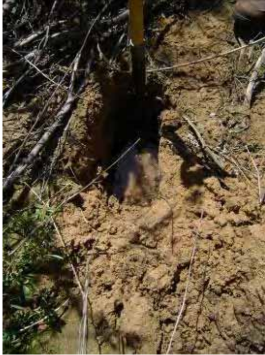
Photo 7. The soil pit dug in Drainage 2 showing thick, saturated sandy soils and a poorly defined upper channel. This pit held several inches of water 5 minutes after digging.
